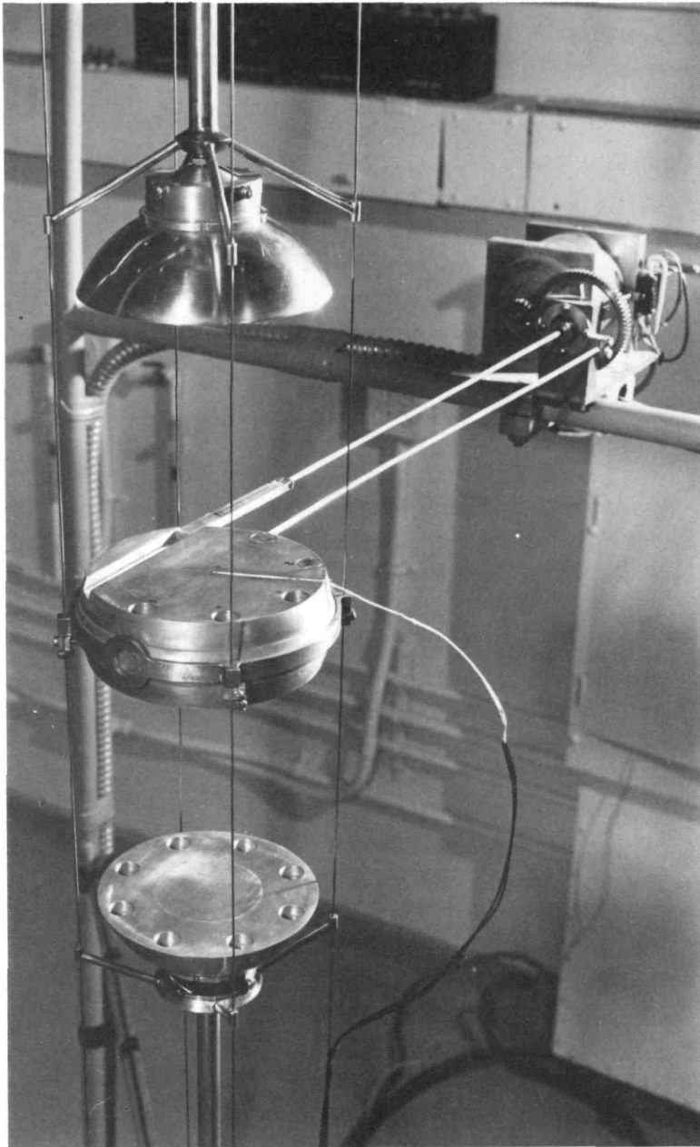
Figure 9 The "Jezebel" assembly. The three large components are placed together to form a sphere when the assembly is operating.
